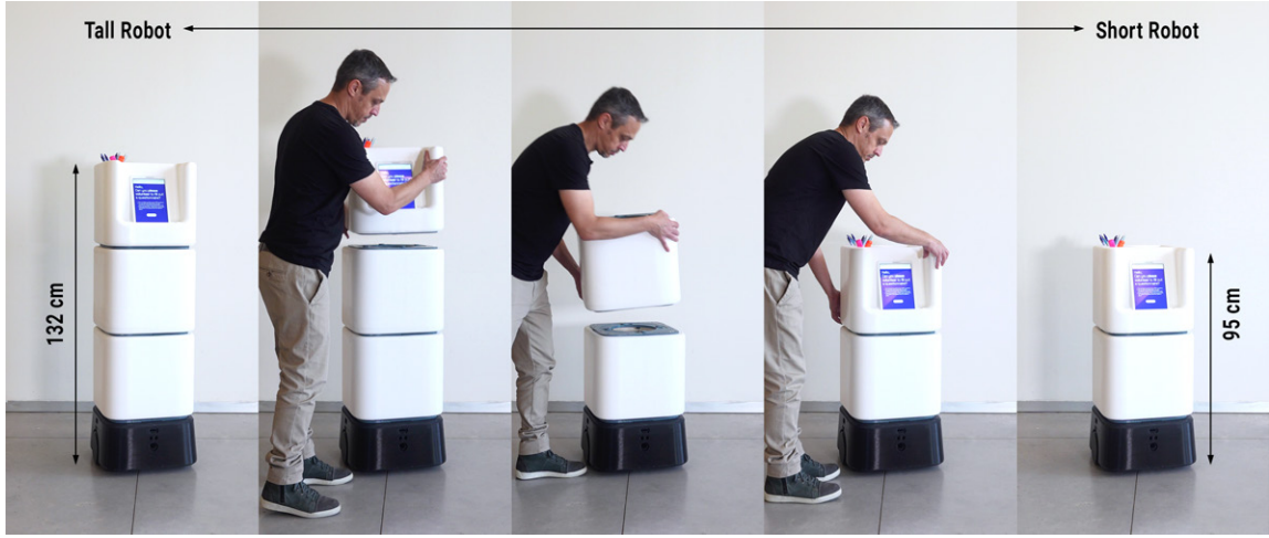
Fig. 2. From Tall to Short, and vice versa. Robot assembly.
